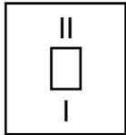
GS2 switch markings - Trickle (I) & Boost (II) Operation
